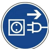
Pull the mains plug before any kind of maintenance and repair work
